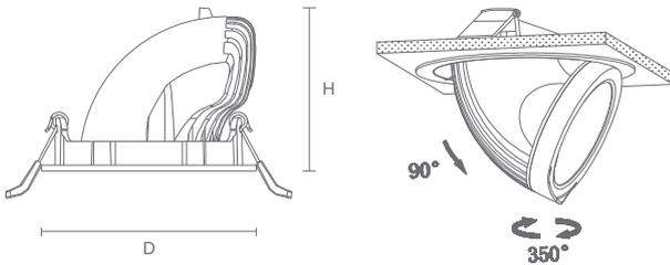
Recess-mounted, COB based multiple zoom light with die cast aluminium housing, anodized reflector and tempered transparent glass diffuser. 40° beam angle.
